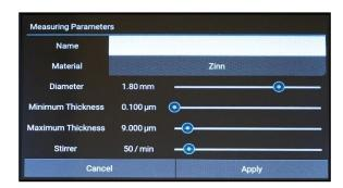
The values can be set either using the sliders or entering the value using an on-screen keyboard. Select type of coating to be examined (AG – SN – NI).
