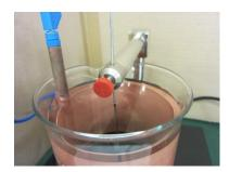
The picture above shows an ideal fixation. Please ensure that the wire does not come into contact with the cathode sheet during the measuring process.
