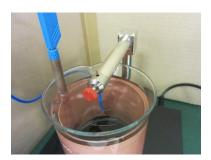
Please ensure that the wire does not come into contact with the cathode sheet during the measuring process.
