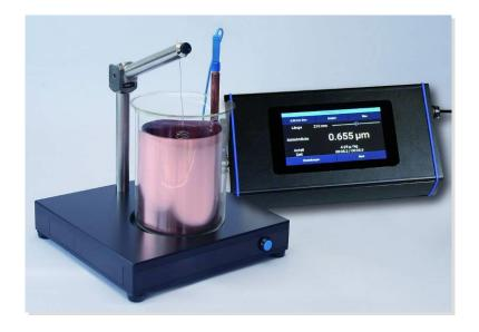
MetaScope 4 is a device used to measure tin, silver and nickel layers on copper wires based on a coulometric technique. The charge required to dissolve the layer in electrolyte is measured and is proportional to the defined wire surface for the layer concerned.
