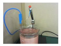
Right after drawing, the material has to be degreased before being put into the beaker (use spirit or the like).
