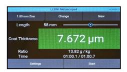
The tin-plating thickness is shown on the display in micrometers Mikrometer (µm).
